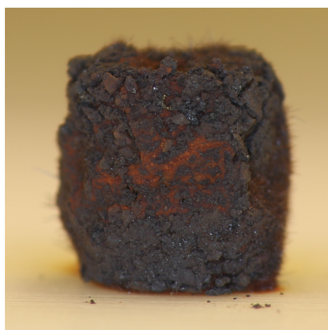
2(c): MnO composite pellet at 1200 °C
